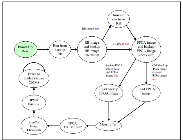
The BIST has been broken down into stages consisting of groups of tests that run at certain times throughout the boot process. The following table shows the different BIST stages and the tests associated with each stage:
